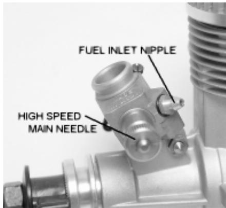
2> Close the carburetor barrel slowly until the lowest possible speed is reached without the engine stopping.
