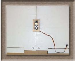
front of the wing, and draw a line around the tray on the surface of the wing. Remove the covering material from within the lines and glue the tray in place. Working through the opening in the tray, use a rotary grinder or hobby knife to cut a hole in the wing surface and the center ribs to clear the servo. Now feed the servo wire between the tray and the wing surface and install the servo with the servo wheel toward the rear, using the directions, which came with the radio.
