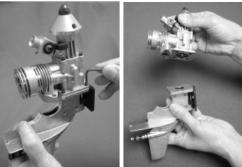
To install muffler, separate the lower unit from the power head by removing the water line and four mounting screws from the power take off mounting plate.
