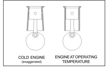
It is also normal for compression to sometimes feel poor when the engine is stopped and turned over while still hot. This is due to the piston cooling faster than the cylinder. If the engine temperature is allowed to stabilize the compression will return to normal.
