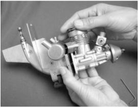
correct direction. Be sure to align the square drive on the flex shaft with the output shaft. Install the four screws loosely but completely into the lower unit thru the PTO (Power Take Off) plate then tighten them. Tighten them in a diagonal fashion. Install the muffler screws and hook up the water pick up line.
