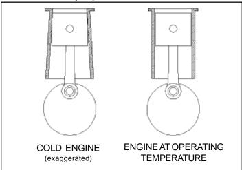
It is also normal for compression to sometimes feel poor when the engine is stopped and turned over while still hot. This is due to the piston cooling faster than the cylinder. If the engine temperature is allowed to stabilize the compression will return to normal.
