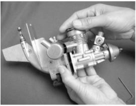
correct direction. Be sure to align the square drive on the flex shaft with the output shaft. Install the four screws loosely but completely into the lower unit thru the PTO (Power Take Off) plate then tighten them. Tighten them in a diagonal fashion. Finally install the muffler screws.
