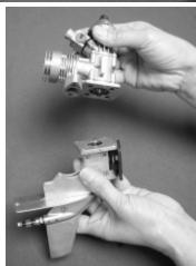
To install muffler, separate the lower unit from the power head by removing the four mounting screws from the power take off mounting plate.
