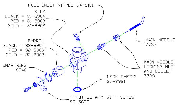
LATE MODEL USES SNAP RING TO RETAIN BARREL
